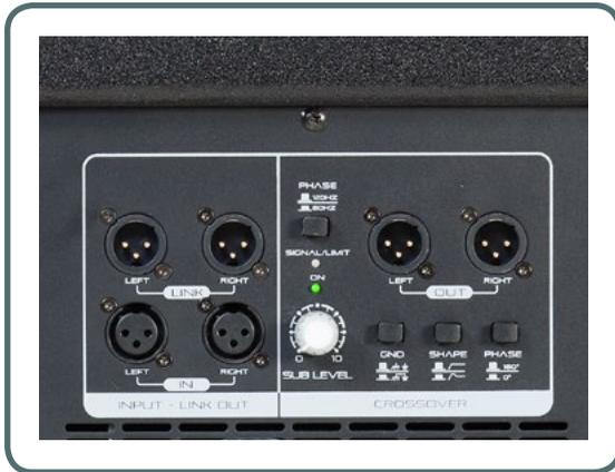
»The powerful and lightweight subwoofers feature electronic stereo crossovers with balanced connections, X-over cut to 80 or 120Hz, phase reverse, filtered and full-range outputs and a few other standard controls. Nothing more simple and essential to complete your PA sound system.
